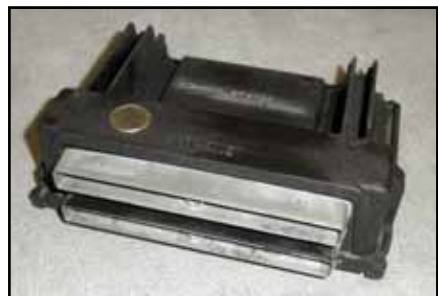
(5) The key ingredient supplied with Nutter's "HemiTronix" deal is a junkyard Delphi computer, used in a bazillion GM cars from 1999 thru 2004. Is this any better than the PCMs used by Ma Mopar? No. But it does have one huge advantage: The aftermarket, apparently with help from the factory, has totally cracked the software code, meaning anyone can tune, modify, calibrate, and tweak to his heart's content.
