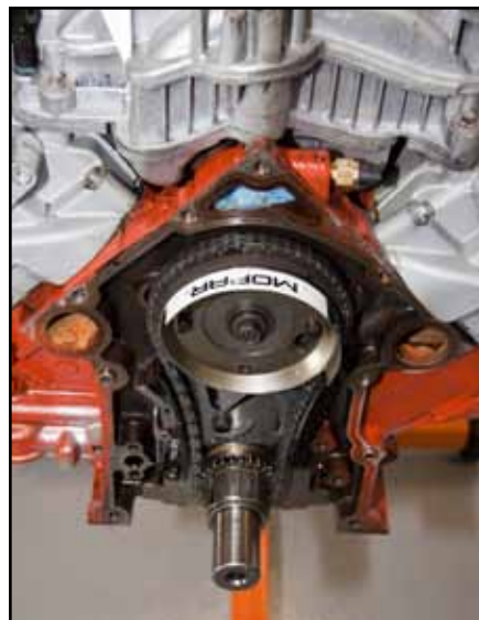
(13) This bolts right onto the camshaft, no gymnastics (and provides an opportunity to install a new timing chain while you are in there).
