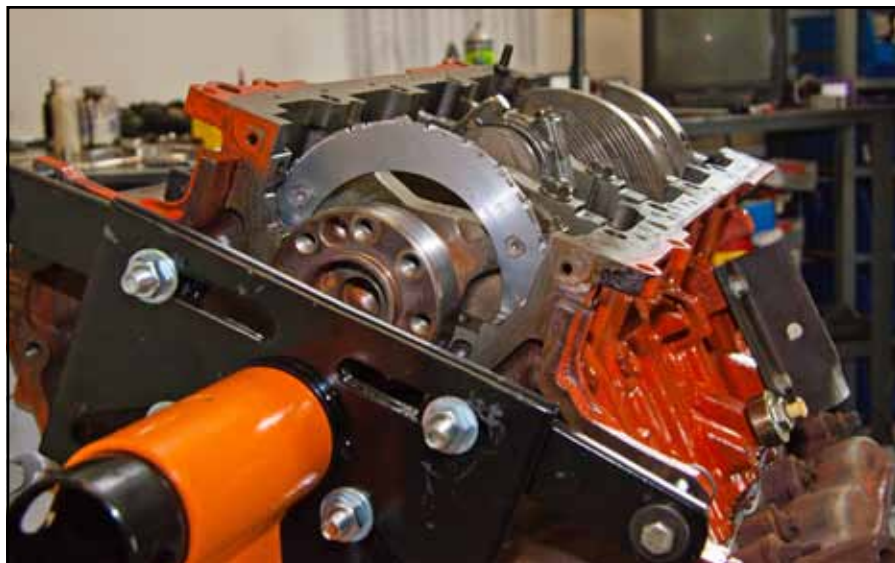
(15) This also bolts on in the stock location. The downside: The crank's gotta come out for this (but the rods, pistons, and cylinder heads can remain in place). Eventually, maybe the Delphi PCM can be taught to read the stock Mopar pulse pattern.
