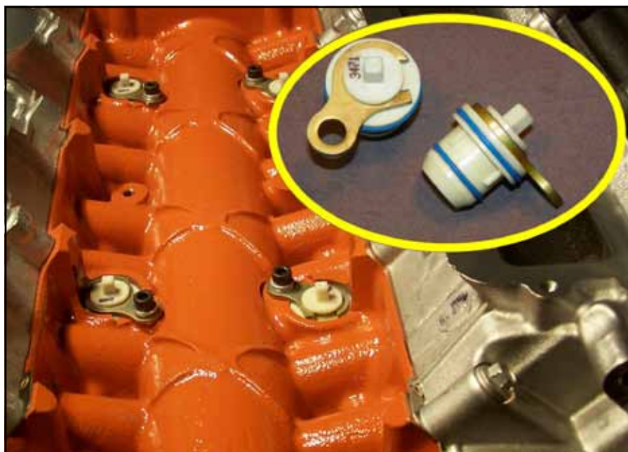
(16) If your engine came with MDS (cylinder deactivation) solenoids, you'd be smart to yank 'em, and replace them with the O-ringed plastic blockoff plugs used on early 5.7L, all 6.1L, and manual-trans 6.4L Hemis. Part number: 53032221AA. They're dirt cheap.
