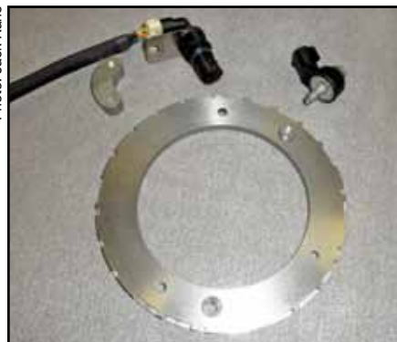
(14) Similarly, a new crank tone ring is included, as is a new detonation sensor (the small gizmo at top right).
