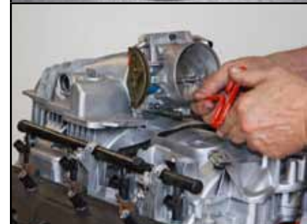
(11) Nutter supplies a huge 80mm hi-flow mechanically-actuated throttle body, complete with matching sensors. It bolts right on to the stock manifold. You will need a longer throttle cable (Lokar, etc.)
