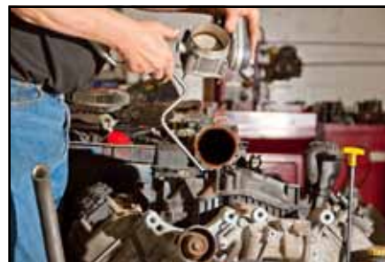
(10) The stock throttle-by-wire body has to go. In its stead...
