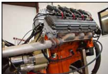
(17) One of the first prototypes ready for a dyno spin. Street? It would be a good idea to use plug wires with boots, and plug the unused plug tubes.
