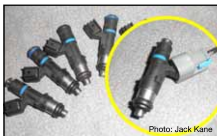
(8) Stock 3G Hemi injectors, including whatever's on your boneyard beast, will plug right into the HemiTronix harness.
