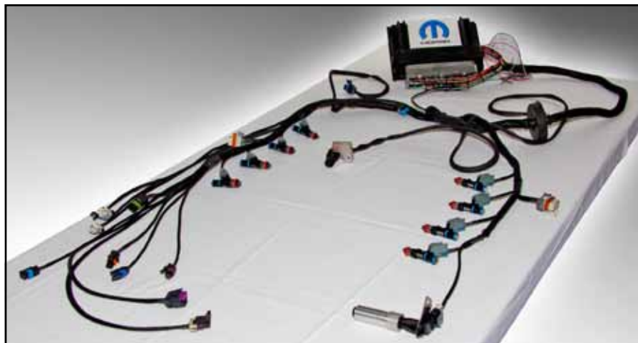
(6) Of course, the Delphi box and Mopar sensors don't normally play in the same sandbox. That's the key to this swap—making the Delphi PCM think it is connected to a GM engine. The primary ingredient in this swap is a custom harness, supplied with the HemiTronix kit. Everything plugs into either the OEM Mopar components (injectors, etc.) or replacement sensors, etc., supplied with the kit. All you have to hook up are, basically, four wires: (1) ground, (2) battery +12V, (3) ignition-on +12V and (4) one wire to the fuel pump.
