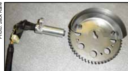
(12) A new cam sprocket with Delphi-compatible cam tone ring (really, just a simple on/off deal, just like what's in a 318 Magnum distributor) is supplied, with a matching sensor and adapter.
